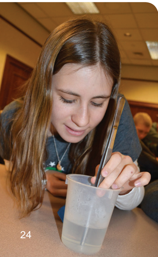
Below: A participant retrieves her NiTiNOL wire, which has reverted to its original shape
